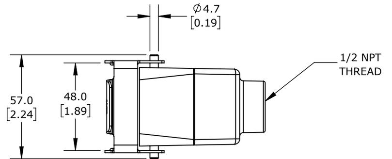
DOUBLE LEVER, TOP ENTRY, CONNECTOR HOUSING SIZE 10B, (1) 1/2 NPT THREADED HOLE, HEAVY-DUTY DIE CAST ALUMINUM. FOR USE WITH METE SIZE 10B 4-PEG CONNECTOR HOUSINGS.
