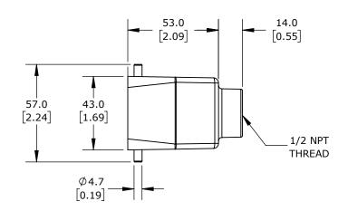
4-PEG, TOP ENTRY, CONNECTOR HOUSING SIZE 10B, (1) 1/2 NPT THREADED HOLE, HEAVY-DUTY DIE CAST ALUMINUM. FOR USE WITH METE SIZE 10B DOUBLE LEVER CONNECTOR HOUSINGS.
