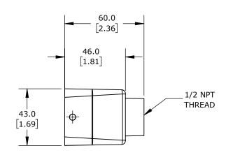
2-PEG, TOP ENTRY, CONNECTOR HOUSING SIZE 6B, (1) 1/2 NPT THREADED HOLE, HEAVY-DUTY DIE CAST ALUMINUM. FOR USE WITH METE SIZE 6B SINGLE LEVER CONNECTOR HOUSINGS.
