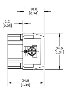
CONNECTOR HOUSING SIZE 16B, 6-POLE, SCREW TERMINALS, ACCEPTS WIRE SIZE 11 AWG, 35 AMP, 600 VAC/VDC, POLES NUMBERED 1 TO 6. FOR USE WITH METE MULTI-WIRE HOUSINGS.
