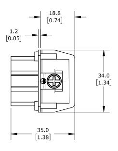
CONNECTOR HOUSING SIZE 16B, 6-POLE, SCREW TERMINALS, ACCEPTS WIRE SIZE 10 AWG, 35 AMP, 600 VAC/VDC, POLES NUMBERED 1 TO 6. FOR USE WITH METE MULTI-WIRE HOUSINGS.
