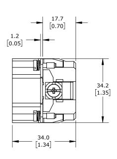
CONNECTOR HOUSING SIZE 6B, 24-POLE, CRIMPED CONTACT, 10 AMP, 600 VAC/VDC, POLES NUMBERED 1 TO 24. FOR USE WITH METE MULTI-WIRE HOUSINGS. REQUIRES 10 AMP MALE CONTACTS METE 14104XXX.
