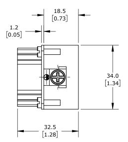
CONNECTOR HOUSING SIZE 6B, 10-POLE, CRIMPED CONTACT, 16 AMP, 600 VAC/VDC, POLES NUMBERED 1 TO 10. FOR USE WITH METE MULTI-WIRE HOUSINGS. REQUIRES 16 AMP MALE CONTACTS METE 14106XXX.
