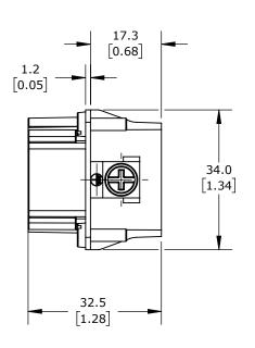
CONNECTOR HOUSING SIZE 6B, 6-POLE, SCREW TERMINALS, ACCEPTS WIRE SIZE 18-14 AWG, 16 AMP, 600 VAC/VDC, POLES NUMBERED 1 TO 6. FOR USE WITH METE MULTI-WIRE HOUSINGS.
