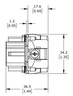
CONNECTOR HOUSING SIZE 6B, 24-POLE, CRIMPED CONTACT, 10 AMP, 600 VAC/VDC, POLES NUMBERED 1 TO 24. FOR USE WITH METE MULTI-WIRE HOUSINGS. REQUIRES 10 AMP FEMALE CONTACTS METE 14103XXX.
