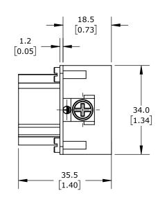
CONNECTOR HOUSING SIZE 6B, 10-POLE, CRIMPED CONTACT, 16 AMP, 600 VAC/VDC, POLES NUMBERED 1 TO 10. FOR USE WITH METE MULTI-WIRE HOUSINGS. REQUIRES 16 AMP FEMALE CONTACTS METE 14105XXX.
