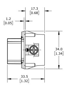
CONNECTOR HOUSING SIZE 6B, 6-POLE, SCREW TERMINALS, ACCEPTS WIRE SIZE 18-14 AWG, 16 AMP, 600 VAC/VDC, POLES NUMBERED 1 TO 6. FOR USE WITH METE MULTI-WIRE HOUSINGS.
