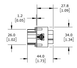
CONNECTOR HOUSING SIZE 24B, 12-POLE, SCREW TERMINALS, ACCEPTS WIRE SIZE 6-16 AWG, 26-14 AWG, 80 AMP (4-POLE), 16 AMP (8-POLE), 600 VAC/VDC, POLES NUMBERED 1 TO 12. FOR USE WITH METE MULTI-WIRE HOUSINGS.
