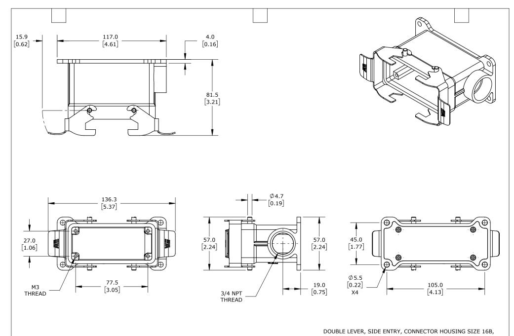
(1) 3/4 NPT THREADED HOLE, HEAVY-DUTY DIE CAST ALUMINUM.
