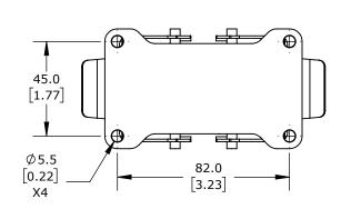
DOUBLE LEVER, SIDE ENTRY, CONNECTOR HOUSING SIZE 10B, (1) 1/2 NPT THREADED HOLE, HEAVY-DUTY DIE CAST ALUMINUM. FOR USE WITH METE SIZE 10B 4-PEG CONNECTOR HOUSINGS.
