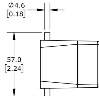
4-PEG, SIDE ENTRY, CONNECTOR HOUSING SIZE 10B, (1) 1/2 NPT THREADED HOLE, HEAVY-DUTY DIE CAST ALUMINUM. FOR USE WITH METE SIZE 10B DOUBLE LEVER CONNECTOR HOUSINGS.
