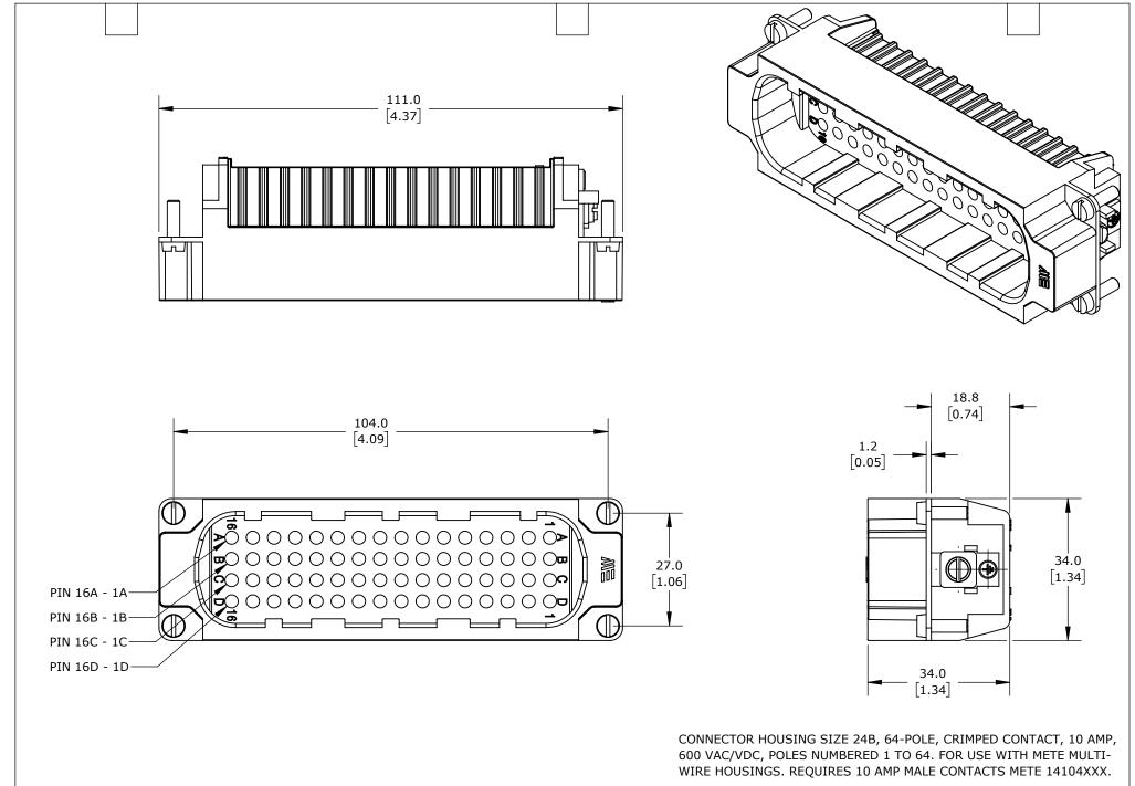
AutomationDirect.com METE MALE INSERT 290253064 1-800-633-0405 UNLESS OTHERWISE NOT TO PART DIMENSIONS MAY DIFFER SLIGHTLY METRIC UNITS USED LATEST VERSION mm SHEET 1 OF 1 ANGLE SCALE FOR PART DESIGN DUE TO MANUFACTURER'S VARIANCES SPECIFIED UNITS ARE: [inch] 2/12/2025
