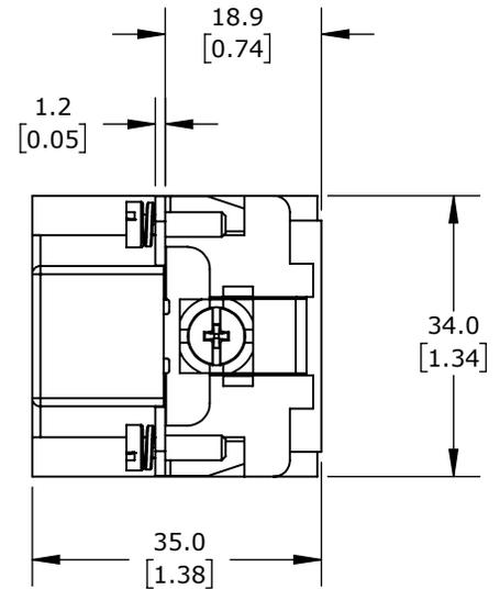
CONNECTOR HOUSING SIZE 16B, 72-POLE, CRIMPED CONTACT, 10 AMP, 600 VAC/VDC, POLES NUMBERED 1 TO 72. FOR USE WITH METE MULTI-WIRE HOUSINGS. REQUIRES 10 AMP MALE CONTACTS METE 14104XXX.
