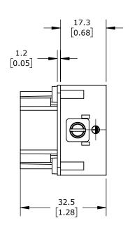
CONNECTOR HOUSING SIZE 16B, 16-POLE, SCREW TERMINALS, ACCEPTS WIRE SIZE 18-14 AWG, 16 AMP, 600 VAC/VDC, POLES NUMBERED 1 TO 16. FOR USE WITH METE MULTI-WIRE HOUSINGS.
