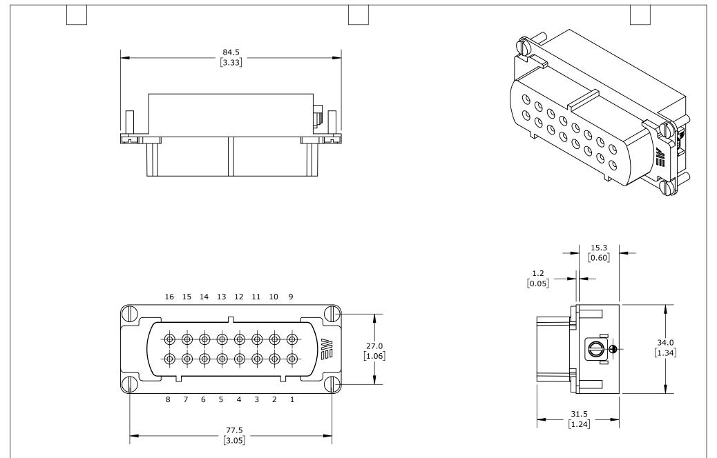
CONNECTOR HOUSING SIZE 16B, 16-POLE, SCREW TERMINALS, ACCEPTS WIRE SIZE 18-14 AWG, 16 AMP, 600 VAC/VDC, POLES NUMBERED 1 TO 16. FOR USE WITH METE MULTI-WIRE HOUSINGS.
