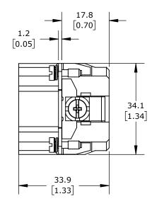
CONNECTOR HOUSING SIZE 10B, 42-POLE, CRIMPED CONTACT, 10 AMP, 600 VAC/VDC, POLES NUMBERED 1 TO 42. FOR USE WITH METE MULTI-WIRE HOUSINGS. REQUIRES 10 AMP MALE CONTACTS METE 14104XXX.
