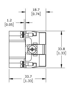
CONNECTOR HOUSING SIZE 10B, 18-POLE, CRIMPED CONTACT, 16 AMP, 600 VAC/VDC, POLES NUMBERED 1 TO 18. FOR USE WITH METE MULTI-WIRE HOUSINGS. REQUIRES 16 AMP MALE CONTACTS METE 14106XXX.
