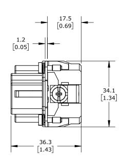
CONNECTOR HOUSING SIZE 10B, 42-POLE, CRIMPED CONTACT, 10 AMP, 600 VAC/VDC, POLES NUMBERED 1 TO 42. FOR USE WITH METE MULTI-WIRE HOUSINGS. REQUIRES 10 AMP FEMALE CONTACTS METE 14103XXX.
