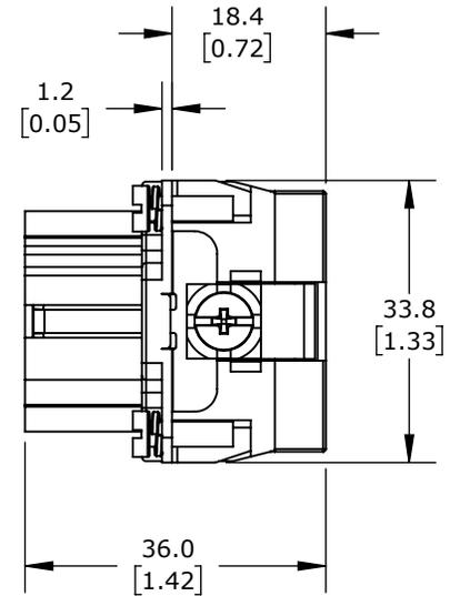
CONNECTOR HOUSING SIZE 10B, 18-POLE, CRIMPED CONTACT, 16 AMP, 600 VAC/VDC, POLES NUMBERED 1 TO 18. FOR USE WITH METE MULTI-WIRE HOUSINGS. REQUIRES 16 AMP FEMALE CONTACTS METE 14105XXX.
