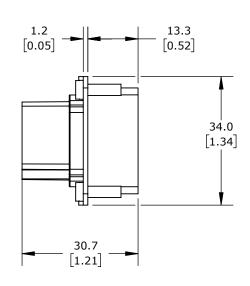
CONNECTOR HOUSING SIZE 10B, 10-POLE, SCREW TERMINALS, ACCEPTS WIRE SIZE 18-14 AWG, 16 AMP, 600 VAC/VDC, POLES NUMBERED 1 TO 10. FOR USE WITH METE MULTI-WIRE HOUSINGS.
