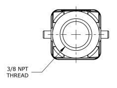
2-PEG, TOP ENTRY, CONNECTOR HOUSING SIZE 3A, (1) 3/8 NPT THREADED HOLE, HEAVY-DUTY DIE CAST ALUMINUM. FOR USE WITH METE SIZE 3A SINGLE LEVER CONNECTOR HOUSINGS WITH MALE INSERTS.
