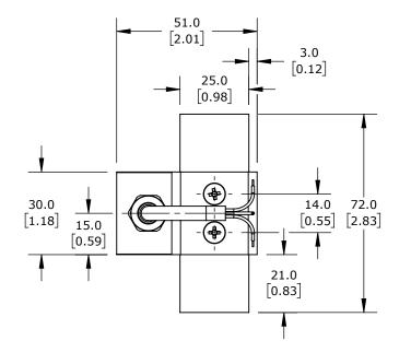
SENSY TENSION AND COMPRESSION LOAD CELL, 66 LB/30 KG, +/- 0.3% OF FULL SCALE ACCURACY, CURRENT SIGNAL RANGE(s) OF 4-20 MA, 10-30 VDC, ANODIZED ALUMINUM ALLOY, IP54, 9.8FT/3M INTEGRAL 4-WIRE SHIELDED CABLE
