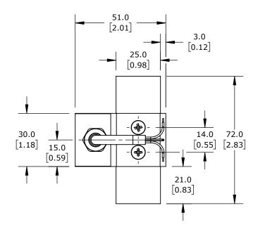
SENSY TENSION AND COMPRESSION LOAD CELL, 440 LB/200 KG, +/- 0.3% OF FULL SCALE ACCURACY, CURRENT SIGNAL RANGE(s) OF 4-20 MA, 10-30 VDC, ANODIZED ALUMINUM ALLOY, IP54, 9.8FT/3M INTEGRAL 4-WIRE SHIELDED CABLE
