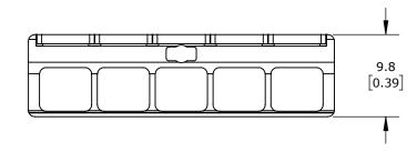
LEVER, SIDE-ENTRY, 5 OPENINGS, COPPER CONDUCTOR, 20-10 AWG SOLID, 20-10 AWG STRANDED, 30A, 600V, POLYCARBONATE HOUSING, TRANSPARENT/ORANGE. PACKAGE OF 15.
