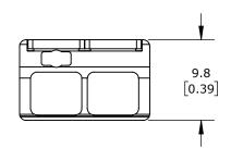
LEVER, SIDE-ENTRY, 2 OPENINGS, COPPER CONDUCTOR, 20-10 AWG SOLID, 20-10 AWG STRANDED, 30A, 600V, POLYCARBONATE HOUSING, TRANSPARENT/ORANGE. PACKAGE OF 50.
