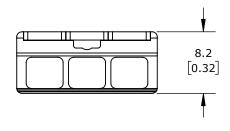
LEVER, SIDE-ENTRY, 3 OPENINGS, COPPER CONDUCTOR, 24-12 AWG SOLID, 24-12 AWG STRANDED, 20A, 600V, POLYCARBONATE HOUSING, TRANSPARENT/ORANGE. PACKAGE OF 50.
