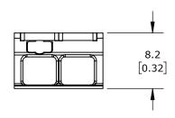
LEVER, SIDE-ENTRY, 2 OPENINGS, COPPER CONDUCTOR, 24-12 AWG SOLID, 24-12 AWG STRANDED, 20A, 600V, POLYCARBONATE HOUSING, TRANSPARENT/ORANGE. PACKAGE OF 100.
