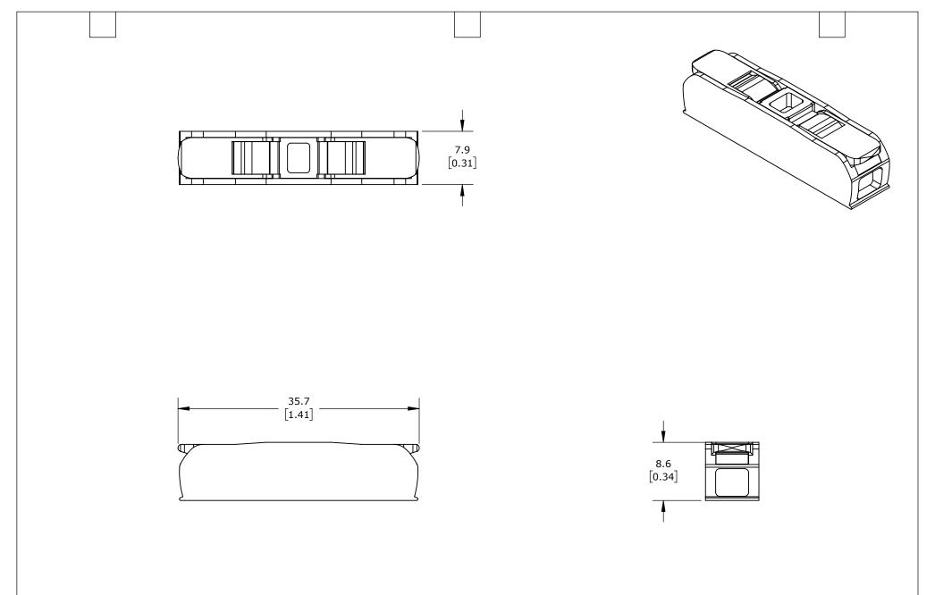
LEVER, IN-LINE, 2 OPENINGS, COPPER CONDUCTOR, 20-12 AWG SOLID, 18-12 AWG STRANDED, 20A, 600V, POLYCARBONATE HOUSING, TRANSPARENT/ORANGE. PACKAGE OF 60.
