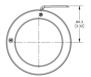
SIFAM TINSLEY AC CURRENT TRANSFORMER, SOLID CORE, 400A PRIMARY, 5A SECONDARY, 4.25IN DIAMETER SENSING WINDOW, +/-1% ACCURACY, 8-32 TERMINAL STUD WITH NUT
