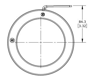
SIFAM TINSLEY AC CURRENT TRANSFORMER, SOLID CORE, 2000A PRIMARY, 5A SECONDARY, 4.25IN DIAMETER SENSING WINDOW, +/- 1% ACCURACY, 8-32 TERMINAL STUD WITH NUT
