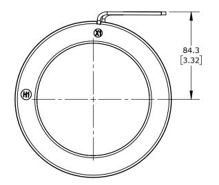
SIFAM TINSLEY AC CURRENT TRANSFORMER, SOLID CORE, 1600A PRIMARY, 5A SECONDARY, 4.25IN DIAMETER SENSING WINDOW, +/- 1% ACCURACY, 8-32 TERMINAL STUD WITH NUT
