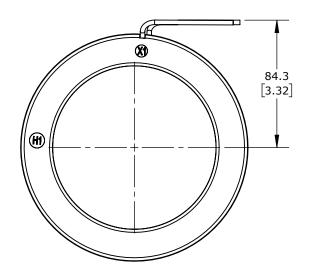
SIFAM TINSLEY AC CURRENT TRANSFORMER, SOLID CORE, 2500A PRIMARY, 5A SECONDARY, 4.25IN DIAMETER SENSING WINDOW, +/- 1% ACCURACY, (2) 24IN 16 AWG LEAD WIRES
