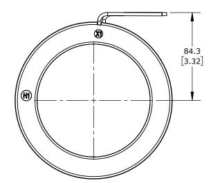
SIFAM TINSLEY AC CURRENT TRANSFORMER, SOLID CORE, 1000A PRIMARY, 5A SECONDARY, 4.25IN DIAMETER SENSING WINDOW, +/- 1% ACCURACY, (2) 24IN 16 AWG LEAD WIRES
