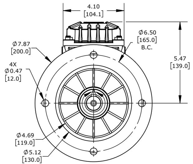
M.G.M. ELECTRIC MOTORS SMX IE3 PREMIUM EFFICIENCY AC INDUCTION MOTOR, GENERAL PURPOSE AND INVERTER RATED, 2HP, 3-PHASE, 230/460 VAC, 1800RPM, TEFC, IEC 90 FRAME, ALUMINUM, D-FLANGE (B5) MOUNT
