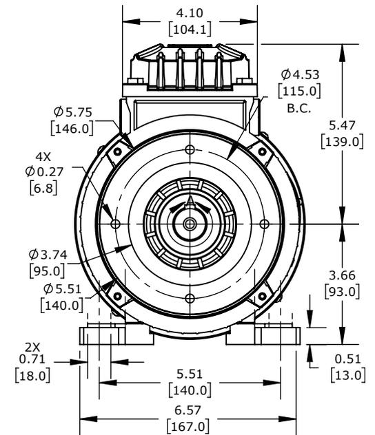
M.G.M. ELECTRIC MOTORS SMX IE3 PREMIUM EFFICIENCY AC INDUCTION MOTOR, GENERAL PURPOSE AND INVERTER RATED, 2HP, 3-PHASE, 230/460 VAC, 1800RPM, TEFC, IEC 90 FRAME, ALUMINUM, C-FACE/REMOVABLE RIGID BASE (B34) MOUNT
