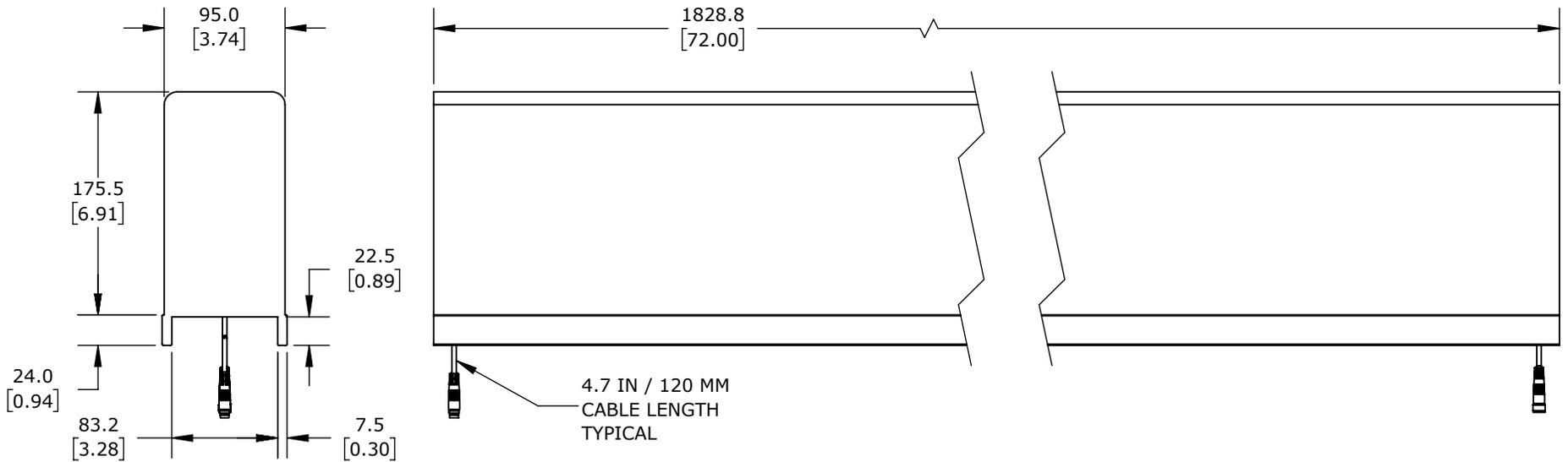
ASO SAFETY SOLUTIONS SAFETY CONTACT BUMPER, 100 X 200MM, 6FT LENGTH, (1) 3-PIN MALE M8 CONNECTOR AND (1) 3-PIN FEMALE M8 CONNECTOR, 4.7IN/120MM CABLE LENGTH. ALUMINUM MOUNTING RAIL INCLUDED.
