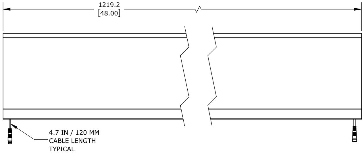
ASO SAFETY SOLUTIONS SAFETY CONTACT BUMPER, 100 X 200MM, 4FT LENGTH, (1) 3-PIN MALE M8 CONNECTOR AND (1) 3-PIN FEMALE M8 CONNECTOR, 4.7IN/120MM CABLE LENGTH. ALUMINUM MOUNTING RAIL INCLUDED.
