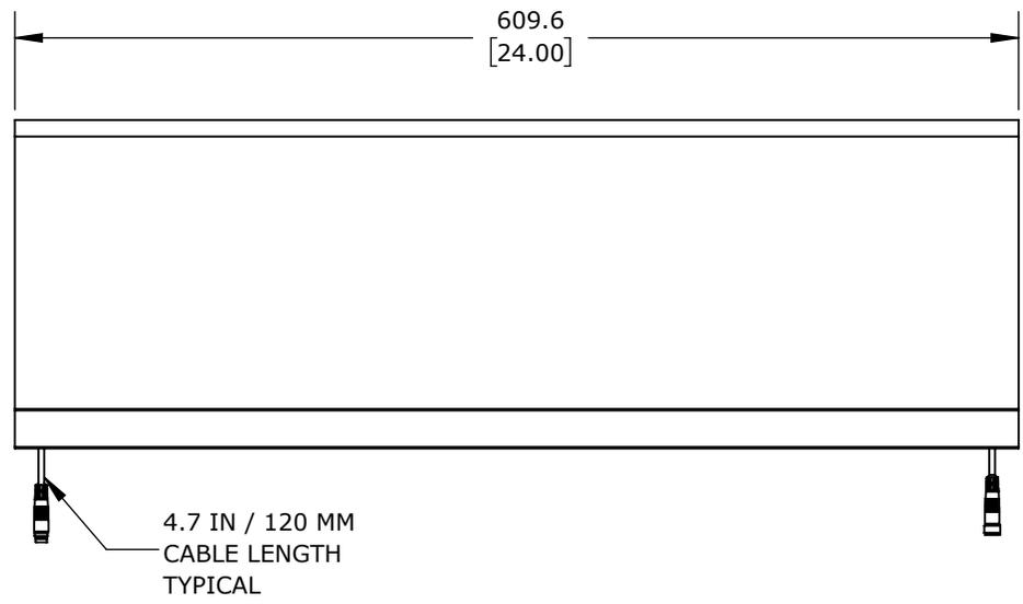
ASO SAFETY SOLUTIONS SAFETY CONTACT BUMPER, 100 X 200MM, 2FT LENGTH, (1) 3-PIN MALE M8 CONNECTOR AND (1) 3-PIN FEMALE M8 CONNECTOR, 4.7IN/120MM CABLE LENGTH. ALUMINUM MOUNTING RAIL INCLUDED.
