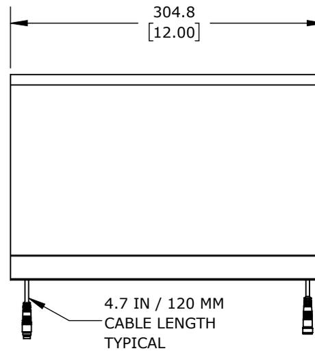
ASO SAFETY SOLUTIONS SAFETY CONTACT BUMPER, 100 X 200MM, 1FT LENGTH, (1) 3-PIN MALE M8 CONNECTOR AND (1) 3-PIN FEMALE M8 CONNECTOR, 4.7IN/120MM CABLE LENGTH. ALUMINUM MOUNTING RAIL INCLUDED.
