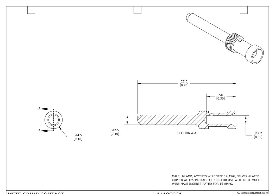
METE CRIMP CONTACT 14106664 1-800-633-0405 UNLESS OTHERWISE NOT TO PART DIMENSIONS MAY DIFFER SLIGHTLY METRIC UNITS USED LATEST VERSION mm SHEET 1 OF 1 ANGLE SCALE FOR PART DESIGN SPECIFIED UNITS ARE: [inch] 3/19/2025 DUE TO MANUFACTURER'S VARIANCES
