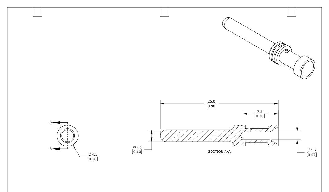
MALE, 16 AMP, ACCEPTS WIRE SIZE 16 AWG, SILVER-PLATED COPPER ALLOY. PACKAGE OF 100. FOR USE WITH METE MULTI-WIRE MALE INSERTS RATED FOR 16 AMPS.
