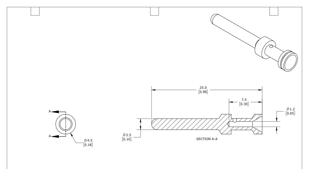
MALE, 16 AMP, ACCEPTS WIRE SIZE 18 AWG, SILVER-PLATED COPPER ALLOY. PACKAGE OF 100. FOR USE WITH METE MULTI-WIRE MALE INSERTS RATED FOR 16 AMPS.
