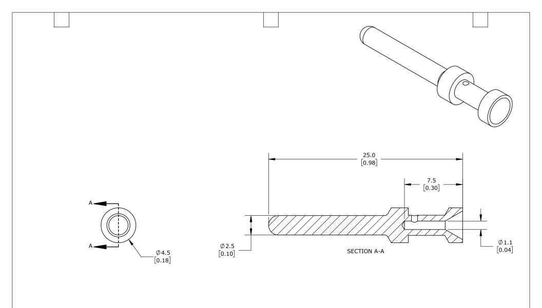
MALE, 16 AMP, ACCEPTS WIRE SIZE 20 AWG, SILVER-PLATED COPPER ALLOY. PACKAGE OF 100. FOR USE WITH METE MULTI-WIRE MALE INSERTS RATED FOR 16 AMPS.
