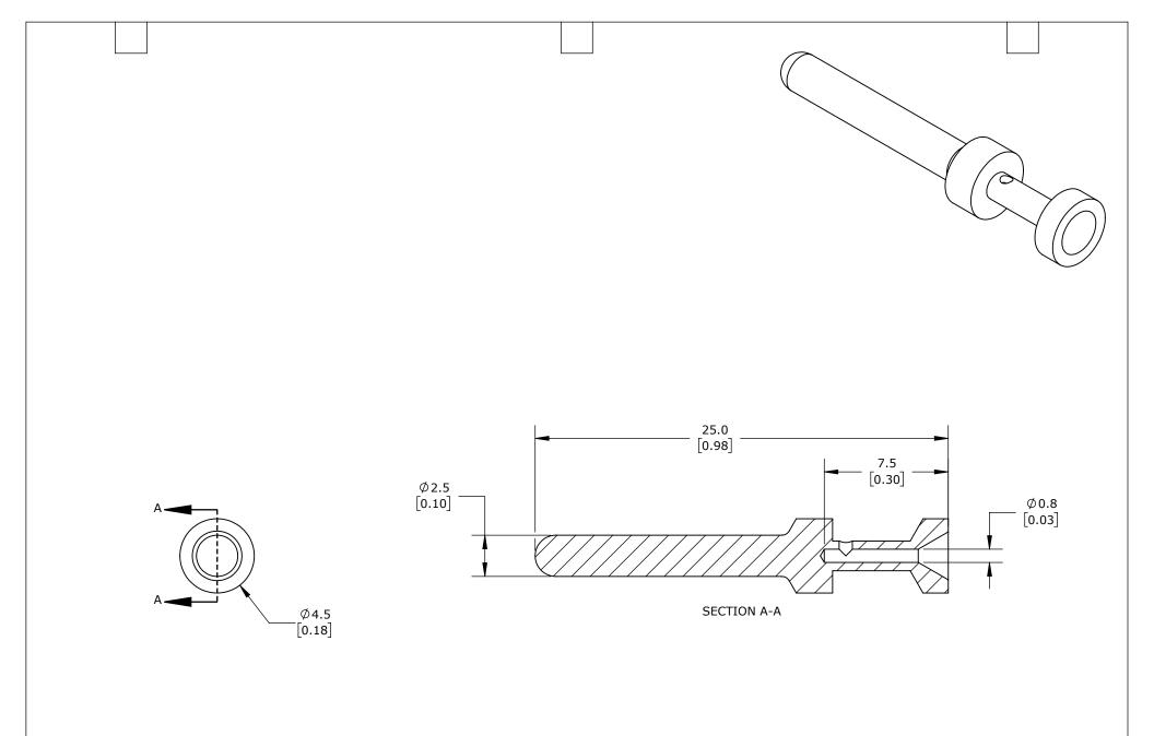
MALE, 16 AMP, ACCEPTS WIRE SIZE 26-22 AWG, SILVER-PLATED COPPER ALLOY. PACKAGE OF 100. FOR USE WITH METE MULTI-WIRE MALE INSERTS RATED FOR 16 AMPS.
