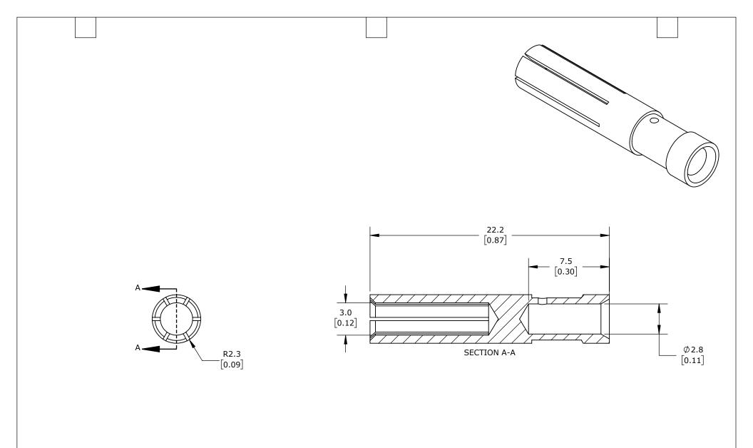
FEMALE, 16 AMP, ACCEPTS WIRE SIZE 12 AWG, SILVER-PLATED COPPER ALLOY. PACKAGE OF 100. FOR USE WITH METE MULTI-WIRE FEMALE INSERTS RATED FOR 16 AMPS.
