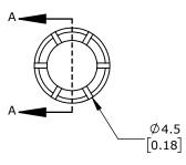
FEMALE, 16 AMP, ACCEPTS WIRE SIZE 14 AWG, SILVER-PLATED COPPER ALLOY. PACKAGE OF 100. FOR USE WITH METE MULTI-WIRE FEMALE INSERTS RATED FOR 16 AMPS.
